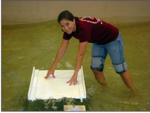
Engineering student in Wave Basin with scale model of the I-10 bridge
