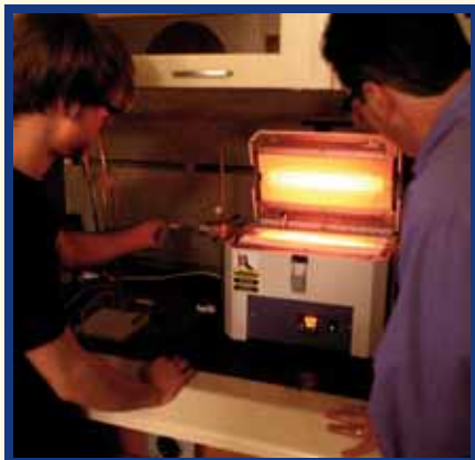
Engineering student Aaron Lepre and Dr. Kevin West oversee the process of converting biofuel by-products into hydrogen for use in fuel cells.
