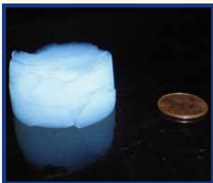
Aerogels are made from the same material as glass, but have a density 100 times lower.
