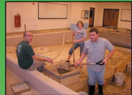
USA CE students sieving the sand in the basin to remove large debris.
