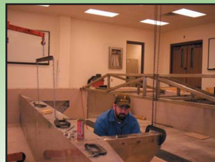
CE student mounting the wave bulkhead to the support frame.
