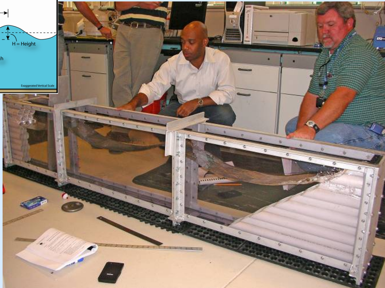
Course participants measuring wave length in the wave flume
