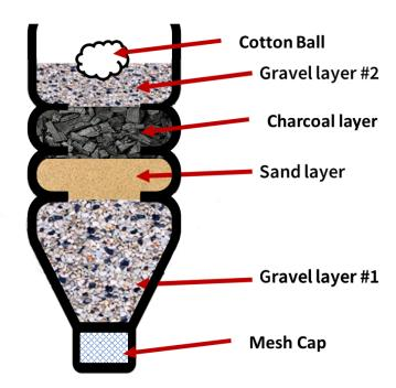
Figure 1: Example Filtration System
