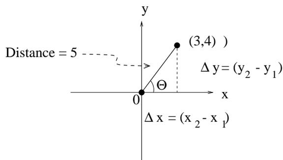
Figure 2.2: The Angle defined by a line
