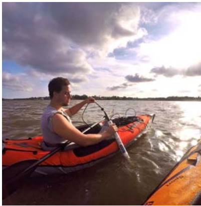
Figure 2: Measuring surface salinity with the Hydrolab Minisonde
